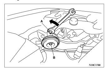
1. Loosen the bolt (A), move the horn (B) (left side only).
